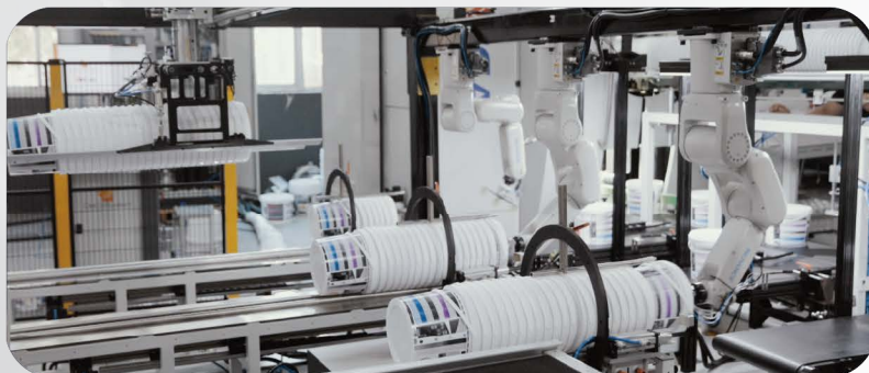
Orientation during pail take off and stacking function
